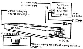
The Charging lamp may not light when a very heavily discharged battery is put on charge. Should this occur, allow several hours to reach a charging condition, as indicated by the Charging lamp. If the battery still cannot be recharged, it will have to be replaced.
